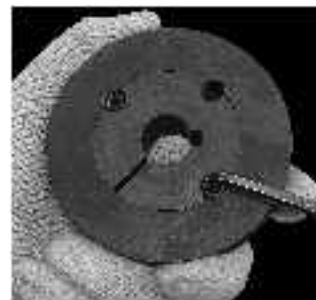
Step 3: Insert the set-screws manually, tighten them with fingers till possible.
