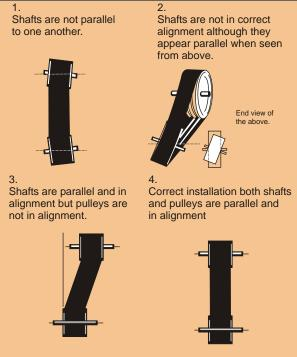
The dotted lines emphasize the faults by indicating the correct position.
